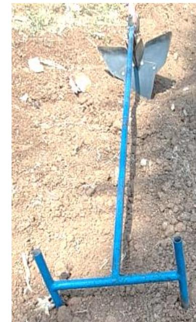
**The pulling type manual weeder is operated by just pulling it over the soil surface.**
