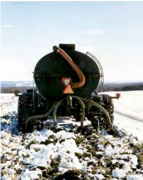
Figure 12.2. Injection of liquid manure into shallow frozen soils, which eliminates compaction concerns and reduces spring application volumes. Photo by Eleanor Jacobs.
