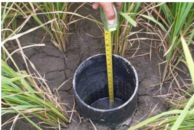
PaniPipes enable farmers to monitor water levels © IRRI
