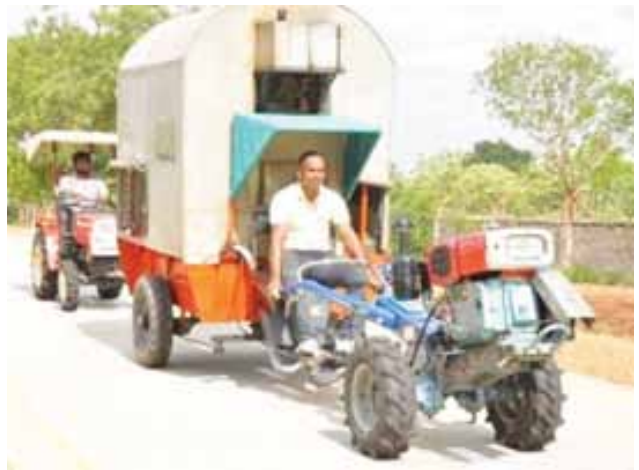
Drawbar Performance Test of Power Tiller
