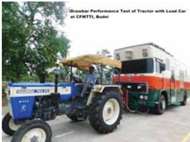
Draw bar Testing of Tractor at CFMTTI,Budni
