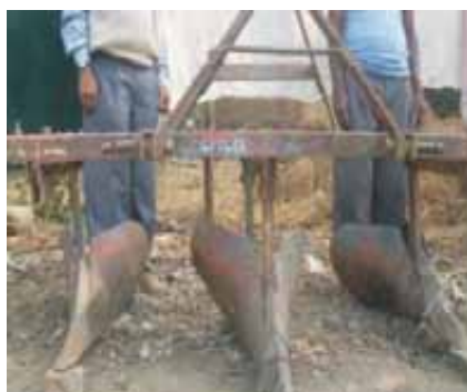
Line /Row Making Innovative implement (Computer) made with iron at Dachamua Village
