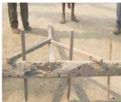
Line /Row Making Innovative implement (Computer) made with wood at Dachamua Village
