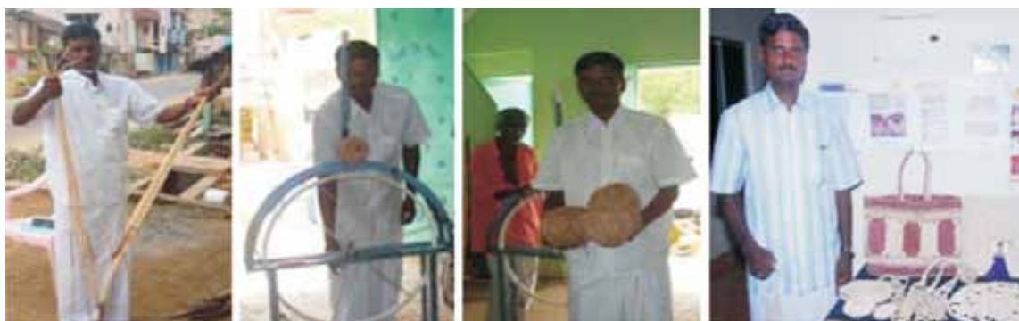
Banana fiber rope making using Murugesan's banana fiber spinning machine
