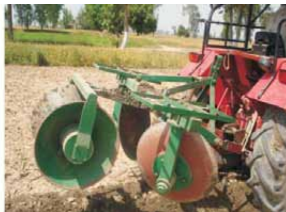
Side view of Disc Bund Maker with pressing roller
