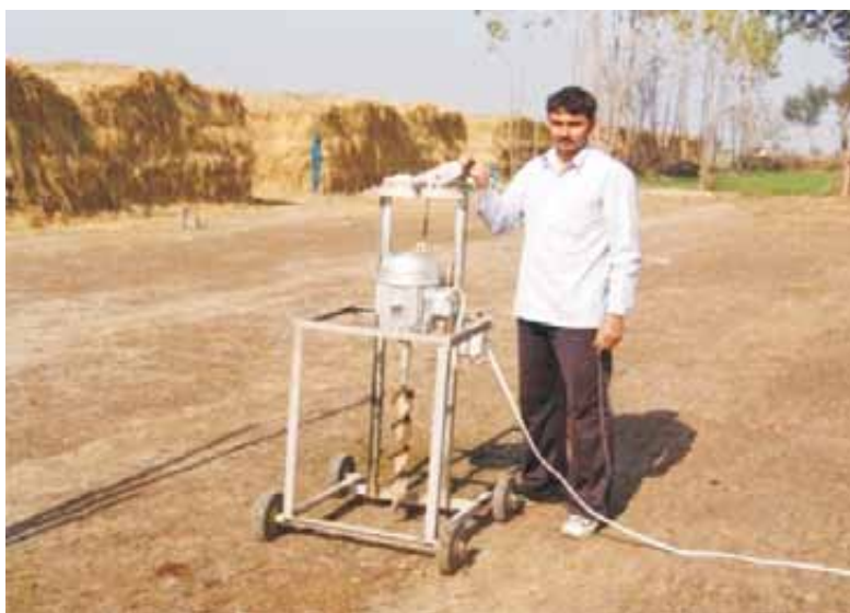
Cost effective improvised hole making machine
