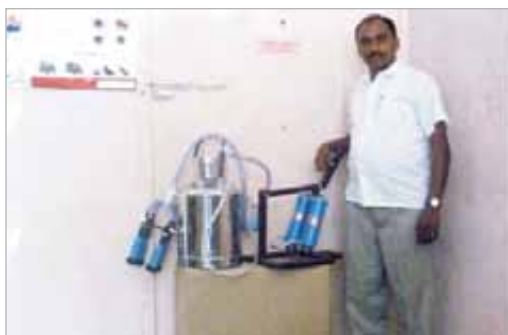
A view of hand operated single cow milking machine ( Valarpirai Milker ) and milking by using it
