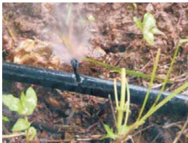
Spraying pattern of Avaran's micro sprinkler
