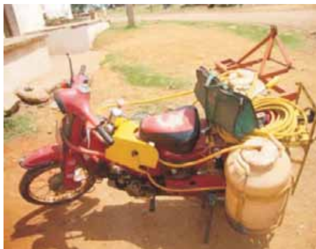
A view of Two Wheeler Mounted Sprayer
