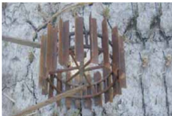
A view of Cage Wheel Type Manual SRI Weeder for Clay Soils
