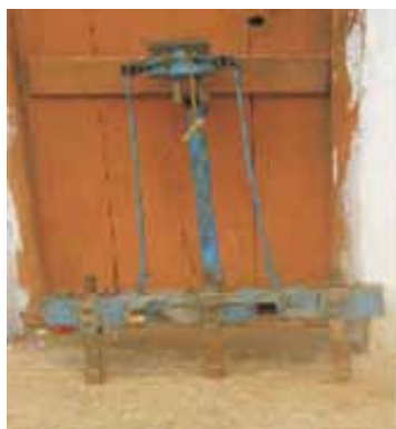
Designed Seed Drill-Cum-Hoe- cum-Weeder
