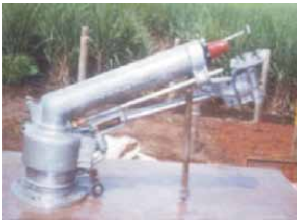
Chandraprabha Rain Gun-Sprinkler System
