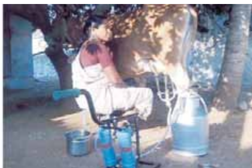
A view of hand operated single cow milking machine ( Valarpirai Milker ) and milking by using it
