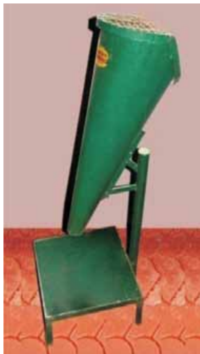
Device for Poly bag filling with potting mixture
