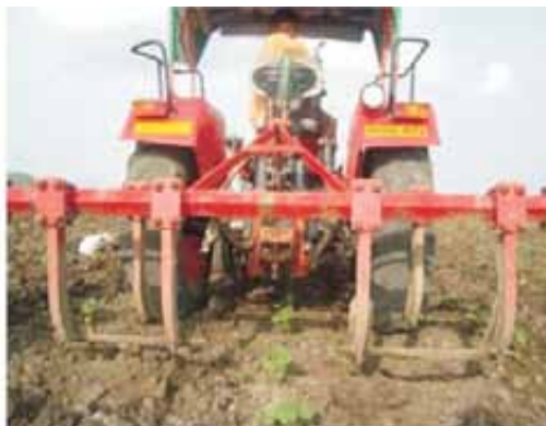
Use of blade in cultivator for weeding
