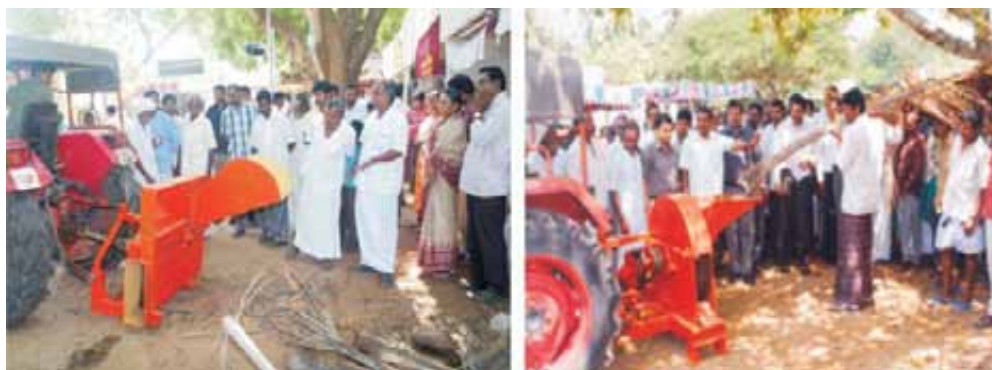
A view of tractor operated farm waste shredder
