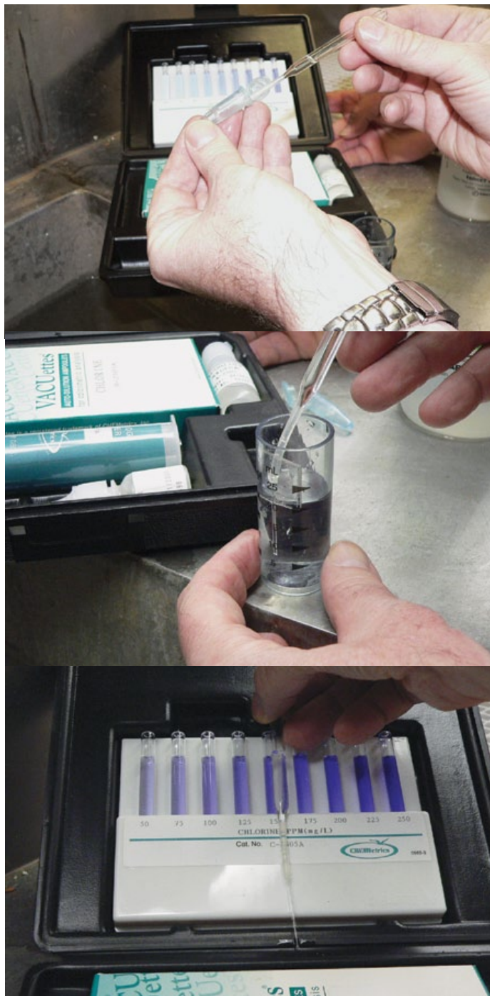
Monitoring dump tank water chlorine levels manually
