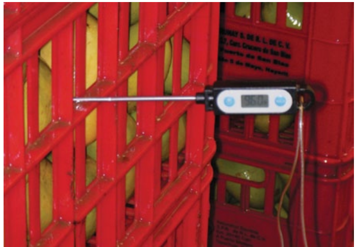
Measuring mango flesh temperature following hydrocooling
