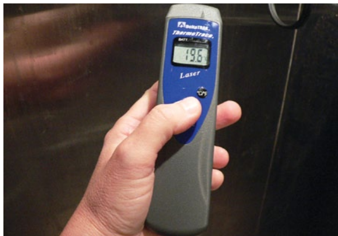
Measuring surface temperature with an infrared thermometer
