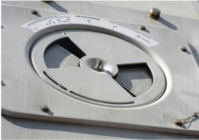
Fresh air exchange on a marine container
