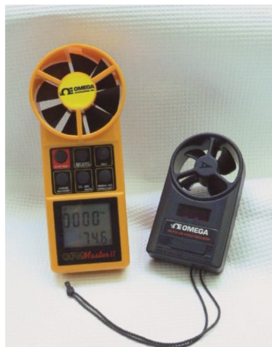
Vane anemometers used to measure air velocity
