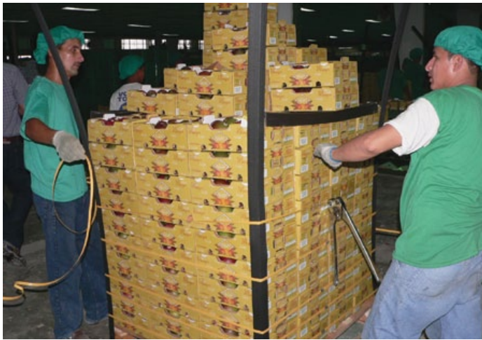
Corner bracing and strapping being applied to a pallet
