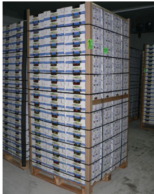
Corner view of a pallet with four-way entry, cartons lined up and within edges of pallet, corner bracing and strapping, and pallet board inserted between carton layers to maintain correct stacking orientation.
