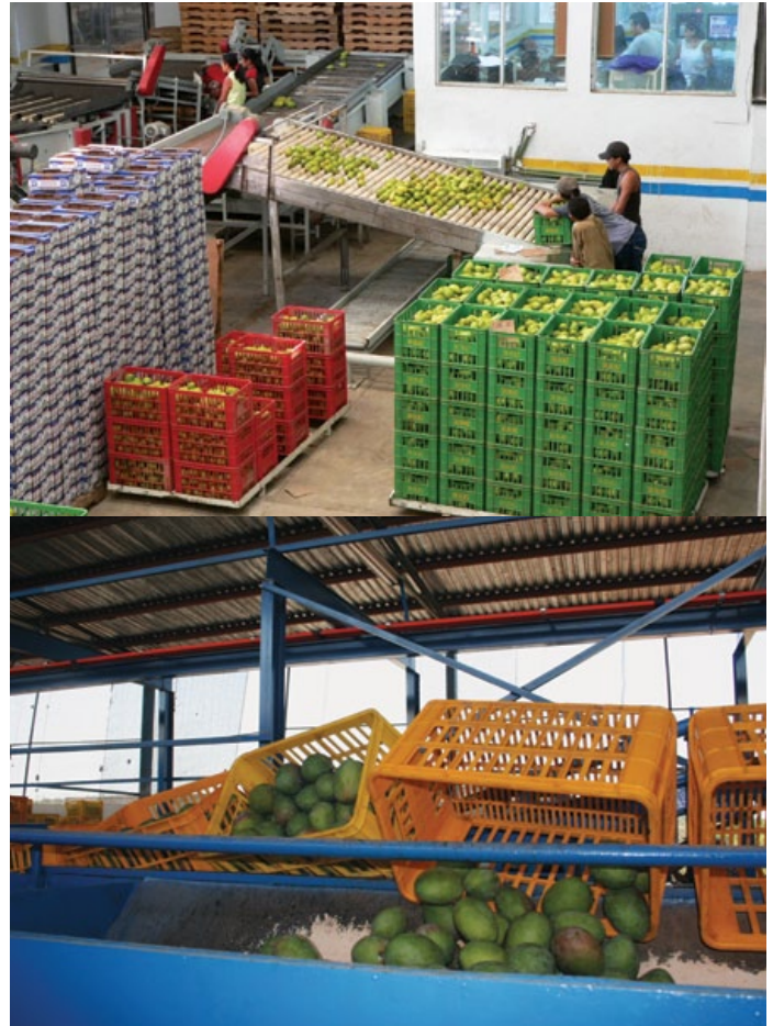
Manual (top) and automated (bottom) dumping of mangos onto a packingline
