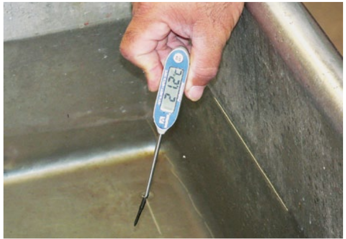
Measuring hydrocooler water temperature
