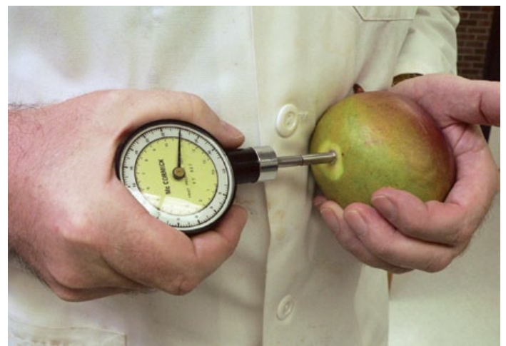
Measuring mango flesh firmness with a penetrometer
