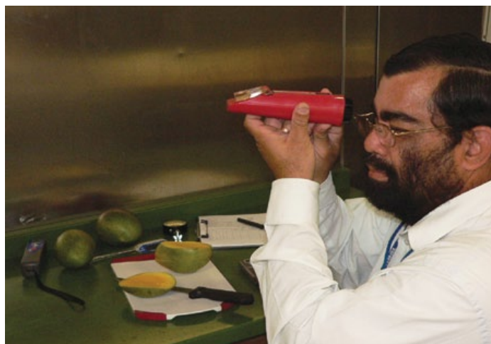
Measuring mango fruit TSS with a refractometer
