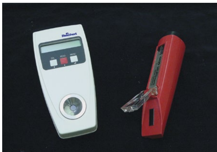
Handheld digital scale (right) and visual scale (left) refractometers
